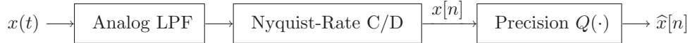
(a) Traditional A/D architecture: Nyquist-rate sampling, followed by fine quantization. The input signal is filtered using an analog anti-aliasing low-pass filter (LPF), and then sampled (C/D) and quantized ( Q(\cdot) ) at the Nyquist rate.
