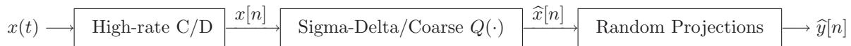
(b) Our proposed Sigma-Delta CS architecture: High-rate sampling, followed by coarse Sigma-Delta quantization and random projections. The Sigma-Delta block architecture is very similar to the classical Sigma-Delta block in Fig. 1(b), and the random projections are implemented in the digital domain.
