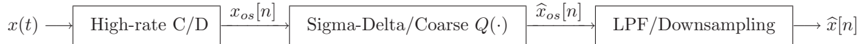
(b) Sigma-Delta A/D architecture: Oversampling, followed by coarse Sigma-Delta quantization. The downsampling and the low-pass filter are implemented in the digital domain.
