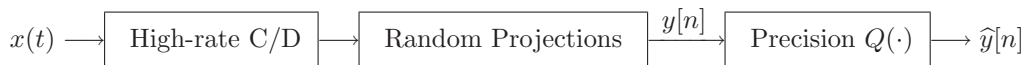
(a) Standard CS architecture: Random projections, implemented in the analog domain, followed by fine quantization.
